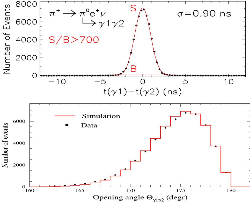
Figure 4: Representative  $\pi_\beta$  decay experimental spectra: signal-to-background ratio (top), and measured and simulated opening angle between the secondary photons produced by the neutral pion from the  $\pi_\beta$  decays (bottom).
