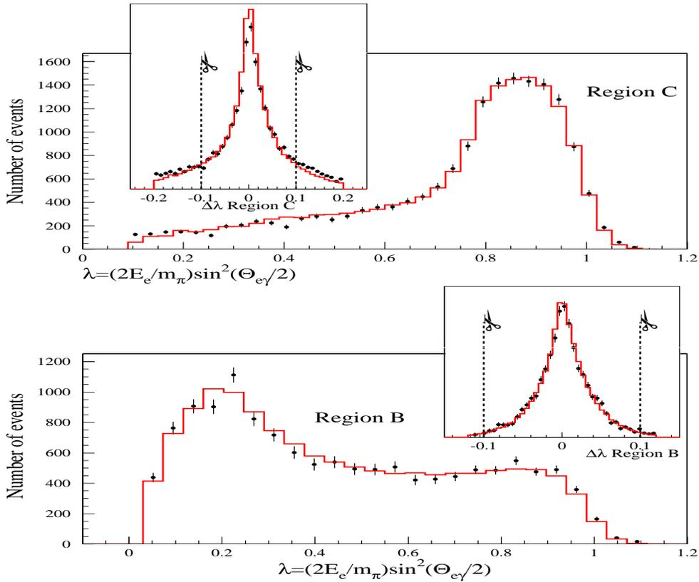
Figure 5: Select spectra for  $\pi^+ \rightarrow e^+\nu_e\gamma$  decay: kinematic variable  $\lambda = 2E_e/m_\pi \sin^2(\theta_{e\gamma}/2)$  which is redundantly measured in our experiment as  $\lambda' = (E_\gamma + E_e - m_\pi/2)/E_\gamma$  for regions C (top) and B (bottom). Inserts show plots of  $\Delta\lambda = \lambda - \lambda'$
