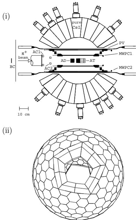
Figure 1. Pibeta detector: (i) cross-sectional view showing the major detector sub-systems, and (ii) 240-module pure CsI calorimeter geometry.
